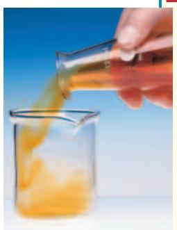
The density of a gas can be used to identify it. This gas is denser than air and can be poured from one container to another.
